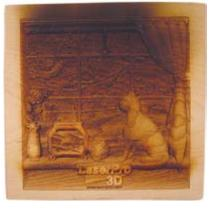
Figure 9: This first attempt at 3-D engraving wood is a reminder that 60 watts is a powerful laser.
