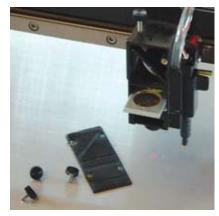
Figure 6: The lens is very easy to clean and replace. A 2" lens comes standard but a 4" lens is optionally available.
