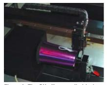
Figure 3: The GX offers a cylindrical attachment as one of its standard accessories.
